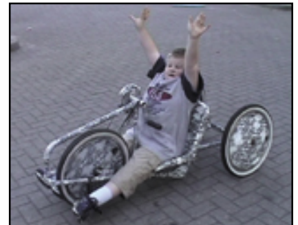
First prototype of Wilson's Tilting Trike is tested by young user
