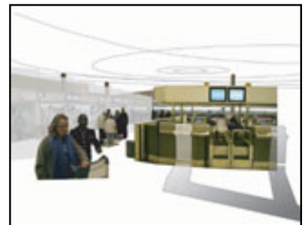
Scene editing at Heathrow to aid orientation: the principle makes use of floor and ceiling markings
